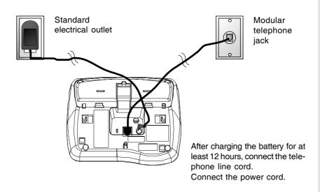
**NOTE:** Install the base unit away from electronic equipment such as personal computers, television sets or microwave ovens. Avoid excessive heat, cold, dust or moisture.
